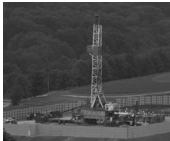
A drilling rig at a Marcellus Shale well site. These drilling rigs are over 100 feet tall. To get a sense of the scale, note how the rig dwarfs the pickup trucks at the far left.
